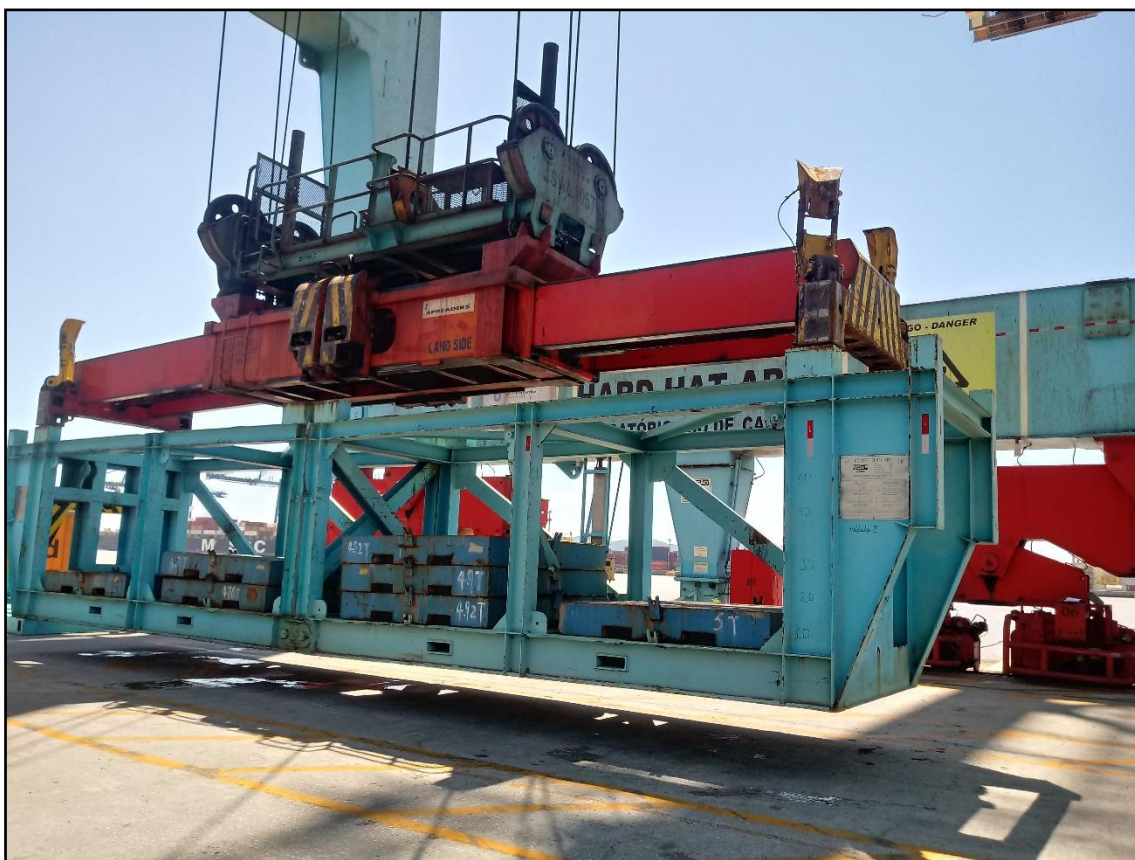
Figura 3. Teste de carga – Single Lift.
