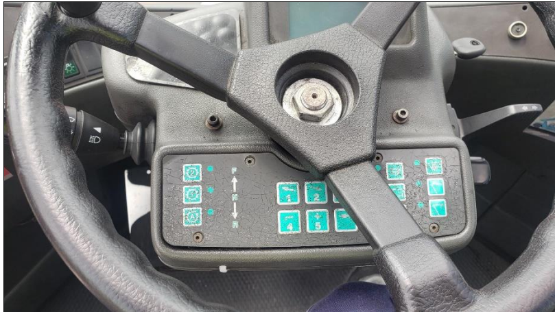
# item 5 – painel com marcas de ressecamento
