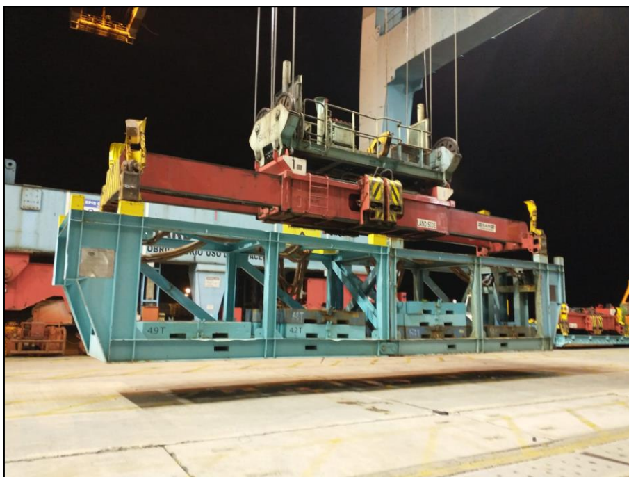
Figura 3. Teste de carga – Single Lift.
