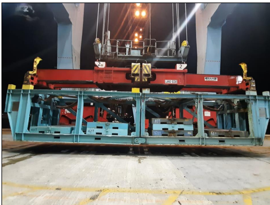
Figura 3. Teste de carga – Single Lift.
