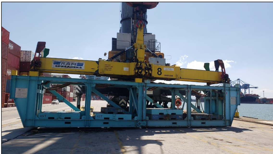
Figura 3. Teste de carga – Single Lift.
